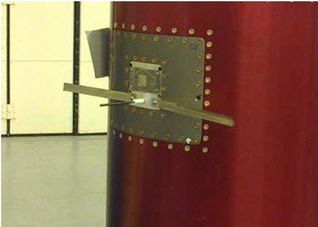
Figure 2 - Langmuir Probe and sounder patch antenna on RSC sounding rocket, June 2014
