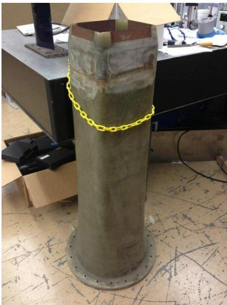
**Figure 1: The existing rectangular exit nozzle**
