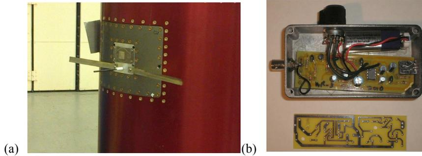
**Figure 4. (a) The WVU Langmuir probe in mission RSC2014 is shown attached to the fuselage of a sounding rocket prior to launch on June 26, 2014. (b) The VLF detector will be miniaturized from a prototype shown.**
