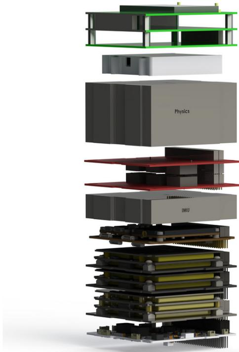
**Figure 6 - STF-1 Component Stack**
