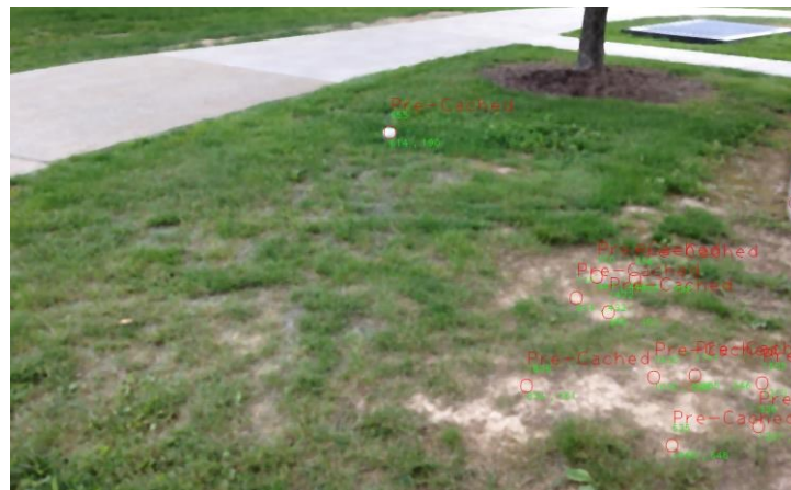
Figure 2 - Resulting candidates from segmentation algorithms. Candidates are circled in red.
