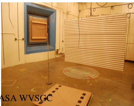
Figure 2: Diffusor panel installed in center configuration, 0°, mounted on swivel
