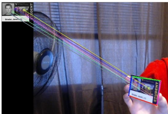
Figure 1 - Successfully detected object using Speeded Up Robust Features (SURF)
